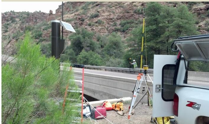
JE Fuller staff performing an RTK (Real-Time Kinematic) GPS survey at Devils Canyon at US Highway 60 near Superior, Arizona
